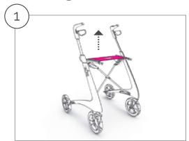
1. Lift the seat by the cut-out in the centre to release the locking mechanism.
