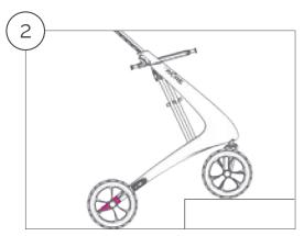
Even though Carbon Ultralight is the world's lightest walker and therefore is easier to lift, it is equipped with a kerb lifter that makes it easier to get over smaller obstacles like kerbs and low steps. This is particularly helpful if heavy objects are transported in a front-mounted basket or bag.
