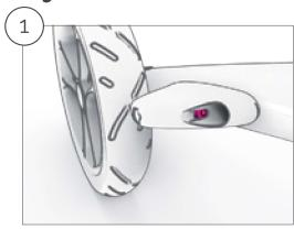
The brake should be adjusted if the brake force applied to the wheel is insufficient (this can occur if the tyres are worn) or the parking brake is difficult to activate (which is most often seen after replacement of a worn down tire). Always set the handle to the desired height before the brake is adjusted as the positon may cause a little variation of the brake adjustment.
