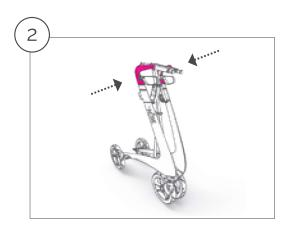
2. To ensure that the rollator is completely folded, push the handles toward each other.
