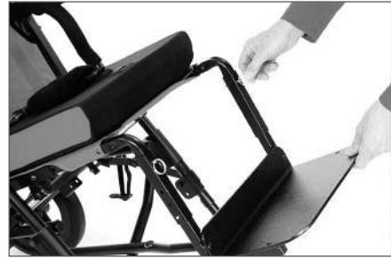
**Step 7** Swing footplates forward, or attach one-piece footplate. **Fig 7**
