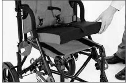
**Step 5** Attach the seat cushion by pushing firmly into the back of seat, then pressing down onto Velcro®. **Fig. 5**
