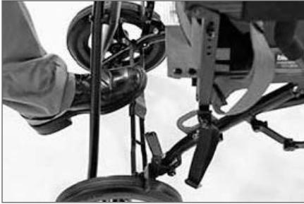
**Step 4** Push down with your foot on therear lock brace until it is in the locked position. **Fig. 4**
