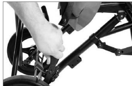
**Step 9** Apply wheel locks before placing individual into chair. **Fig. 9**
