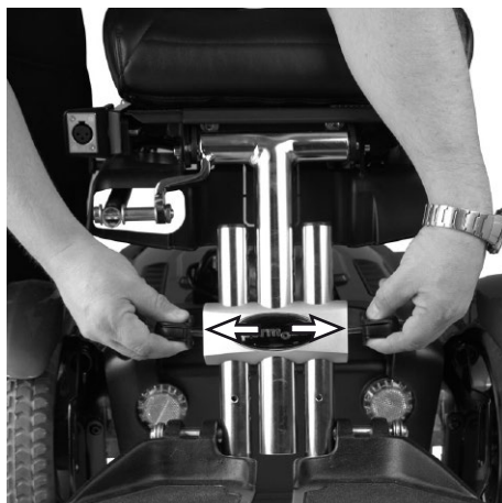
Locking pins for height adjustment of the leg rest.
