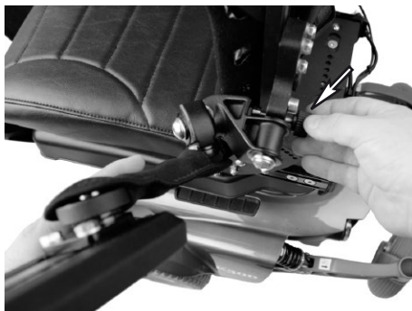
Adjustment knob for angling the arm rest.
