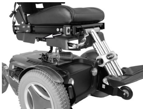
Spring-lock pin for the leg rest angle.
