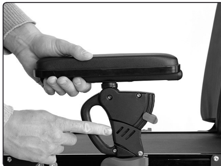
Adjustment of arm rest height
