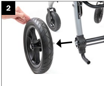
2. Grasp wheel and pull laterally.
