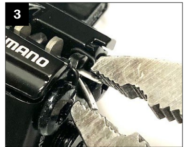
3. Remove cotter pin with pliers.
