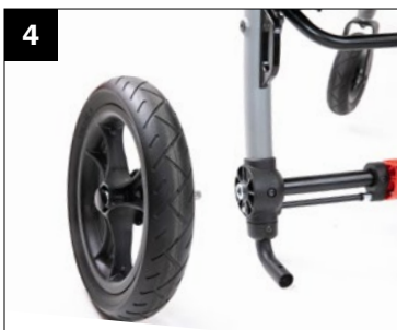
4. Align axle to wheel lock bar.
