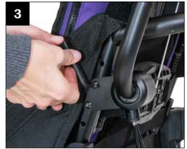
3. If required for additional height adjustment, unscrew the bolt holding the back positioner hardware onto the frame.
