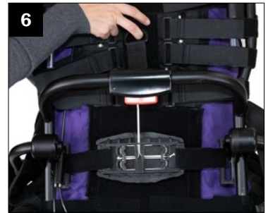
6. Adjust the tension towards the user's back by pulling upward on the tab and hook securely to the back of the tension adjustable back upholstery at the appropriate tension level.
