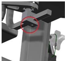
Loosen the set screw located under the block (beneath the footrest) (**fig. 3b**). Slide sideways to the desired width and then retighten with the Allen key. For angle adjustment of the footrest, use the adjustable lever (**fig. 3d**). To do this you will need to lift the lever slightly and then turn clockwise to tighten and counter-clockwise (by raising it) to reposition the lever in the proper place. Rotate the footrest plate to the desired position and retighten.
