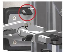
Slide knee supports to the required dimension and retighten securely. For angle adjustment of the knee supports, you will need to lift the lever slightly and then turn clockwise to tighten and counter-clockwise (by raising it) to reposition the lever in the proper place (**fig. 4d**).
