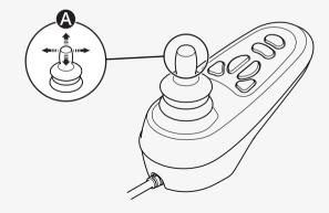
Do not move the joystick before, during, or immediately after you turn on the control system. If you move the joystick during this time, it can generate a joystick error. If this happens, turn off and then on the wheelchair.
